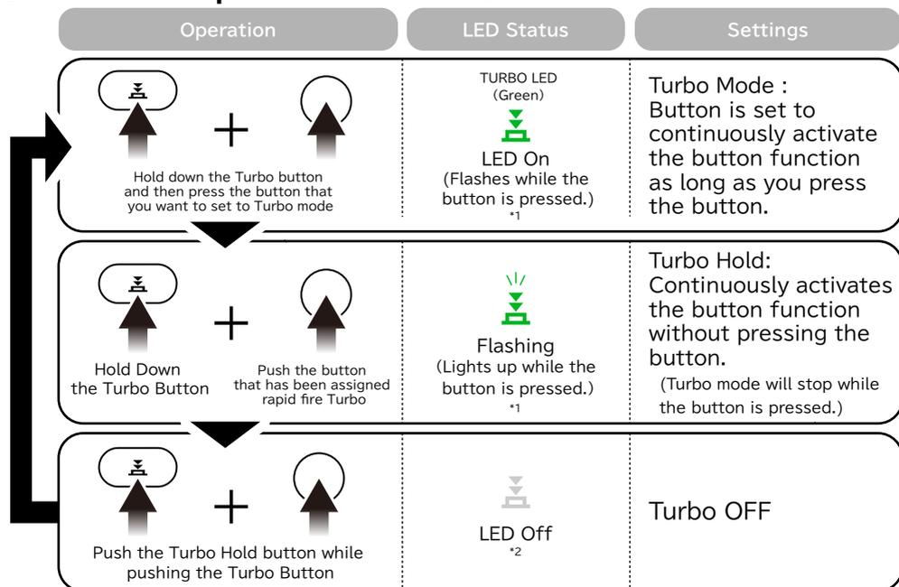
\*1 The Turbo LED (Green) will flash at a rate corresponding to the Turbo speed.
