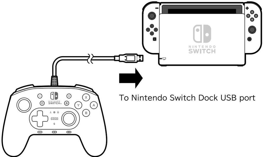
\* Do not touch the Left Analog Stick / Right Analog Stick or any other button when connecting the USB plug.
